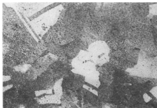
Fig. 2. Levelling of grains when copper was deposited on polycrystalline copper from sulphate bath containing 10 -8 mol dm -3 of DTE at 7.5 mA cm -2 (×625).
